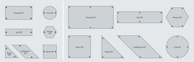
The location of the screws can vary depending on the pattern and substructure when using 300mm Modules.
